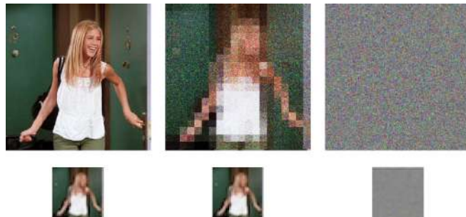
Fig. 1: Left: the original image with its thumbnail. Middle: the TPE-encrypted image with its thumbnail. Right: traditionally encrypted image with its thumbnail.
